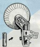
battery (Ever-Ready B155 or equivalent is preferred, but B145 is suitable), so that the positive pole (+) is at the top. Insert the positive end of the battery first. The tape within the body should be underneath the battery, so that when the battery is exhausted it can be removed by lifting the end of the tape. Replace the metal cover and secure it by tightening the knurled locking screw.
